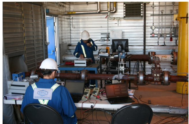
Pressure and Vibration Data acquisition system, including orifice testing
