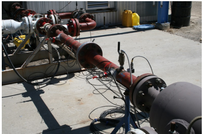
Pulsation generator, above left and pulsation bottle, lower right
