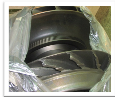
Centrifugal Compressor Damaged During Surge Event
