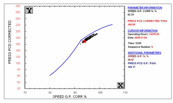
The most likely cause of this problem is inlet guide vane linkage malfunction (looseness or "hanging up").
