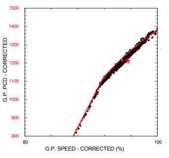
The pressure and temperature deviation is used to determine the optimal maintenance interval. The figure below illustrates multiple blade washing activities. In each case the pressure and temperature is reduced. The deviation starts to increase until the next wash cycle.
