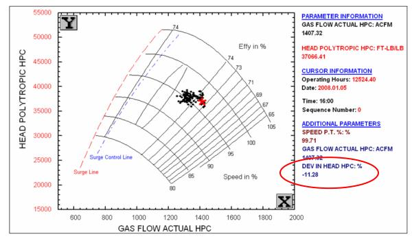
BETA monitors the compressor's performance to detect changes in performance. The wheel curve is one of our analytical tools that is tracked regularly.
