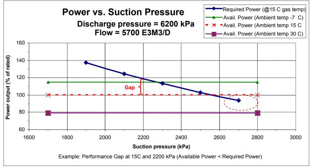
These results were used to investigate various power upgrade possibilities for the gas turbine – an ongoing analysis.
