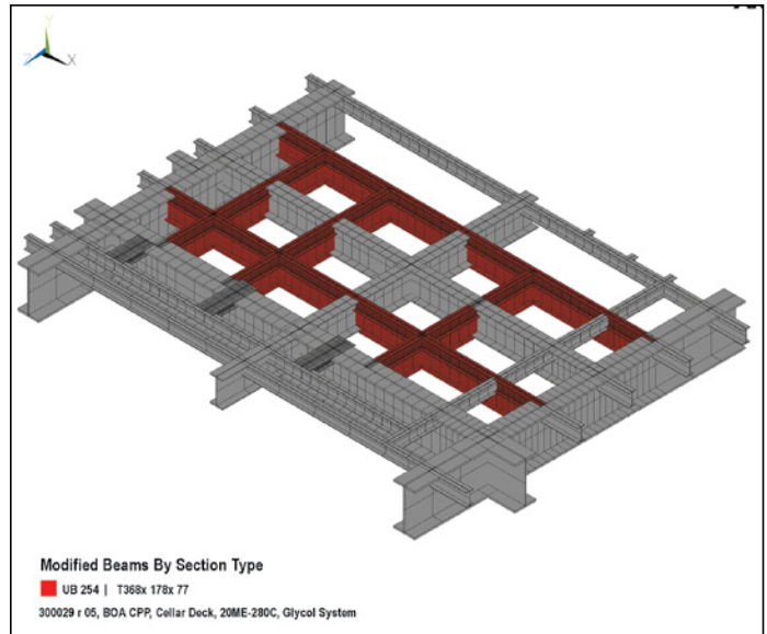
Figure 3: Key beams requiring stiffening.
