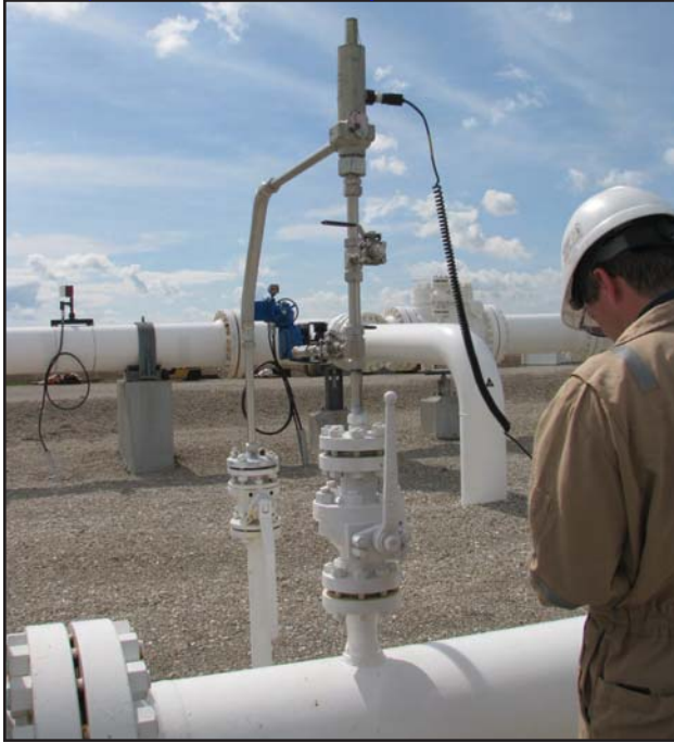
A Beta Machinery Analysis field engineer performing an SBP vibration study.
