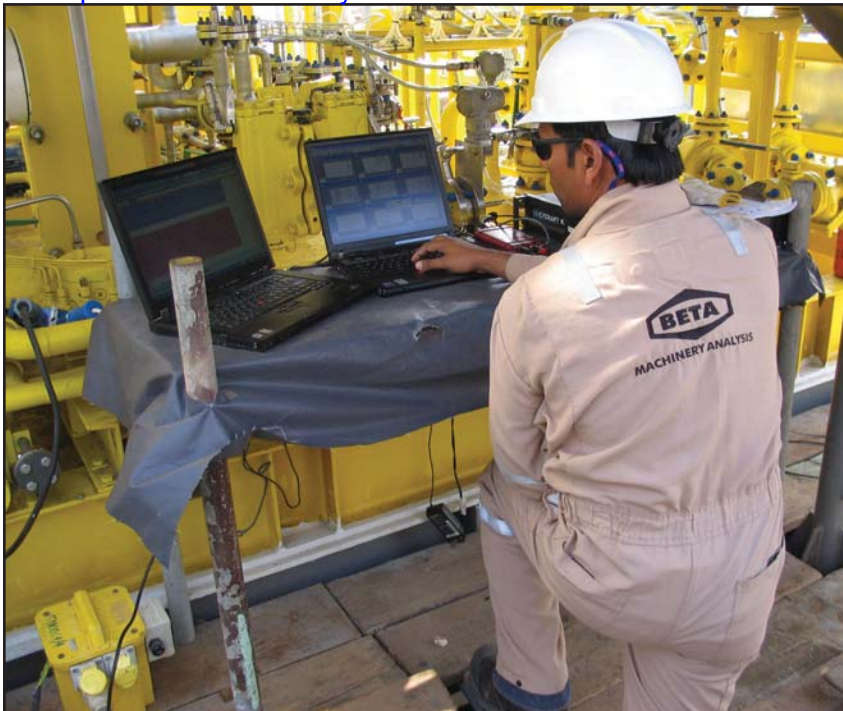
A field engineer performs a vibration audit, including small-bore piping (SBP), at a facility in Abu Dhabi.
