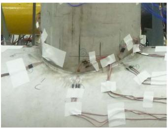
Figure 3: Stub-on tee (NPS 12x20)
