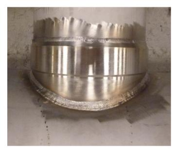
Figure 6: Buttweld Pipet tee (NPS 12x20)
