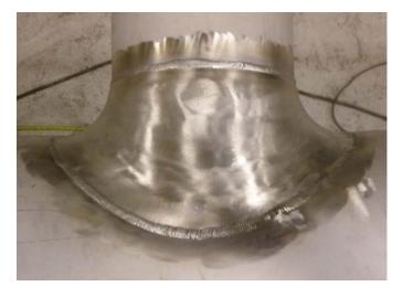
**Figure 5:** Sweepolet tee (NPS 12x20)
