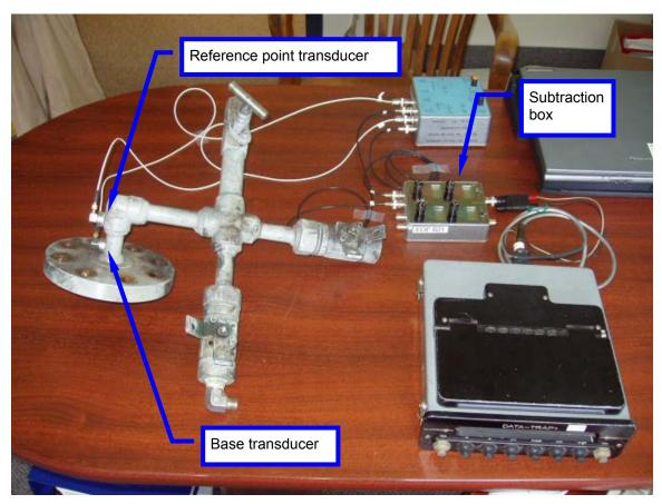
Figure 10. Analysis Setup to Measure Relative Vibration between Base and Reference Point
