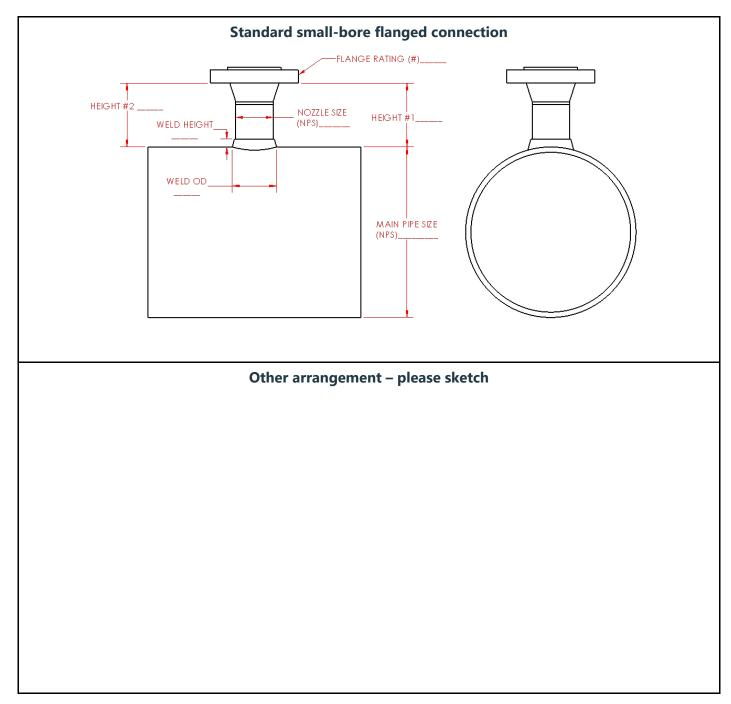
Dimensions provided above form the basis for cutting the DamperX Fins to fit your application. Accuracy in these dimensions is critical. Although some adjustment is possible in the field, inaccurate dimensions may result in poor fitment.
