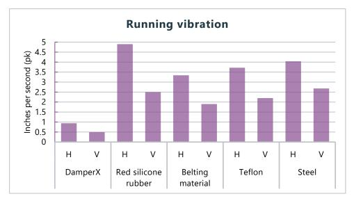
Figure 4 – Running vibration by lining
