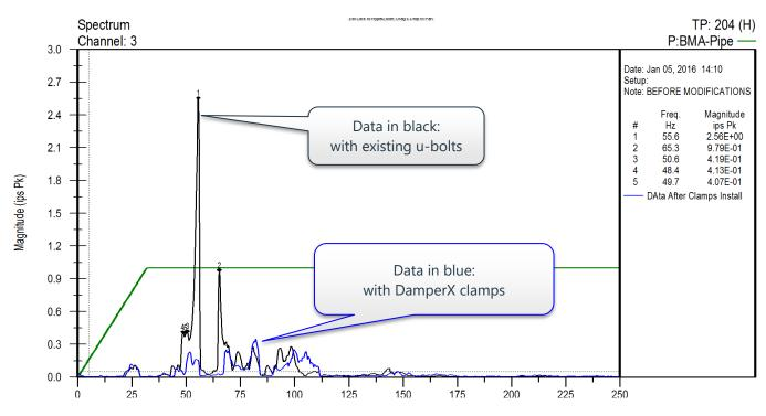
Figure 10 – Operating vibration of main discharge pipe horizontal direction (before and after TP #204)
