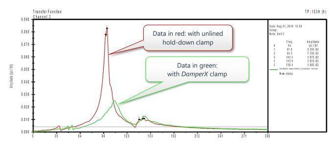
Figure 7 – Impact test of main discharge pipe horizontal direction (before and after TP #103)
