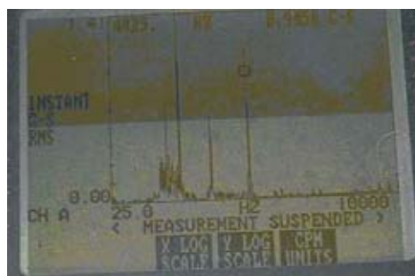
Picture 5: Vibrations at 6H with magnet mount
