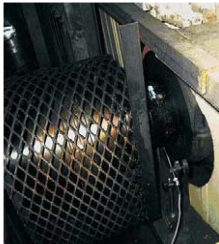
Picture 3: Optical pickup on the low speed shaft. Once per turn mark was put on the shaft while it was running.
