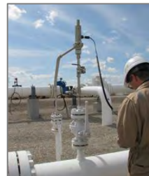
A vibration audit of small bore attachments highlights high risk locations
