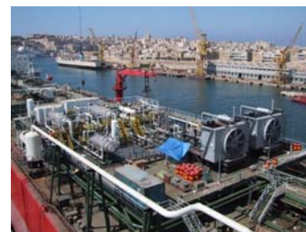
Figure 7: FPSO Design for Two 1000HP (746kW) Compressor Units on a Common Topside Structure
