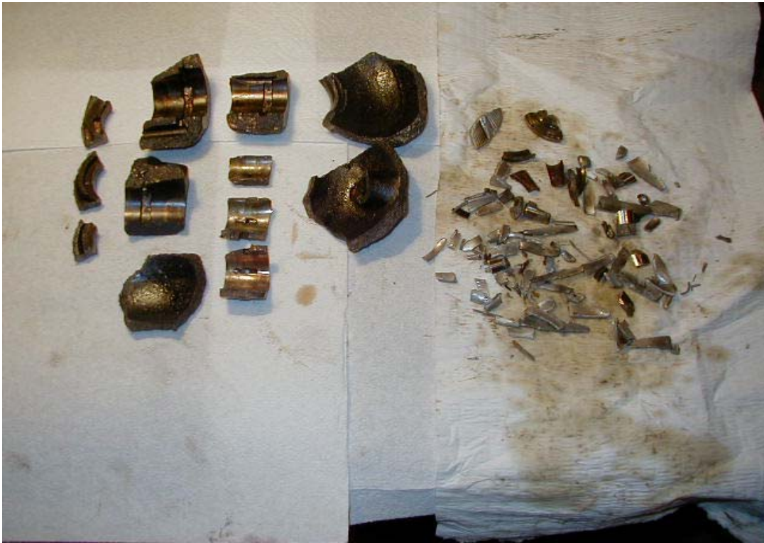
Figure 6 – Failed Turbo Casing and Other Bits
