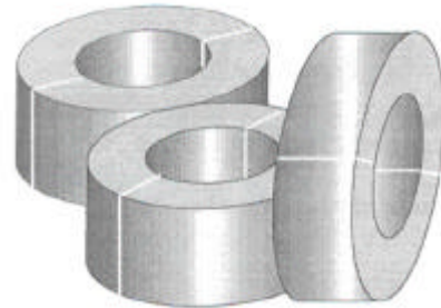
Figure 3. Three donuts added to the compressor shaft solved the problem.
