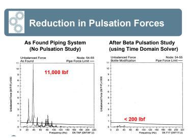
Figure 2.1: Example of Pulsation Forces (before and after a BETA Study)
