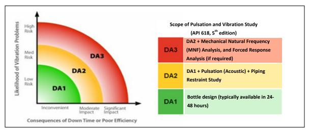
Figure 1.5: Risk Assessment Used to Determine Vibration Design Approach (DA) for the Compressor and Piping System
