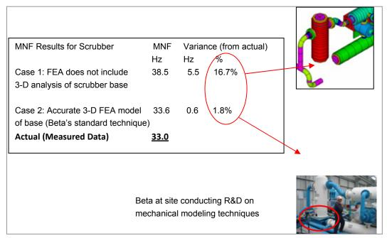
Figure 3.9: FEA Models Must Be Accurate
