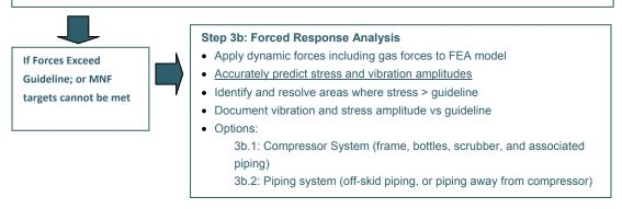
Figure 3.3: Flowchart for DA3 (API 618, 5<sup>th</sup> Ed)
