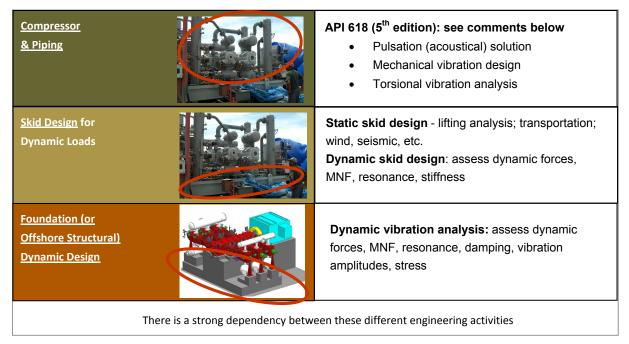
Figure 1.4: Integrated Vibration Design
