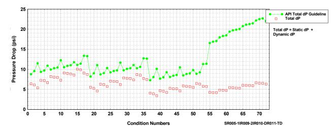
Figure 2.2: Example of Total Pressure Drop Guideline
