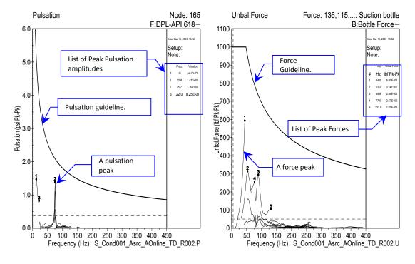
Figure 2.4: Example of Pulsation (Pressure) and Force Plots
