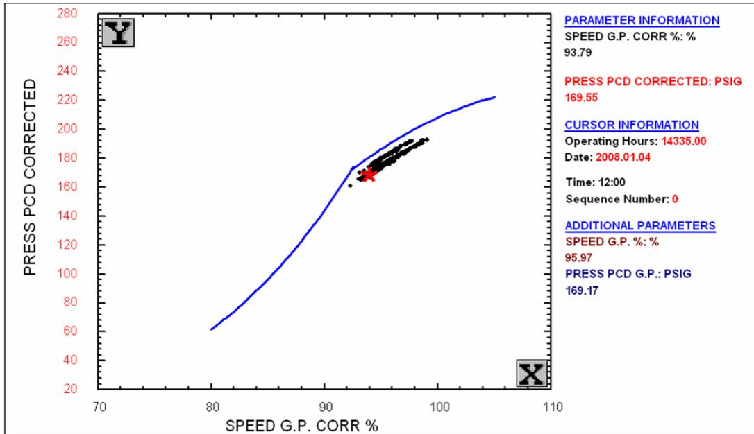
The most likely cause of this problem is inlet guide vane linkage malfunction (looseness or "hanging up").
