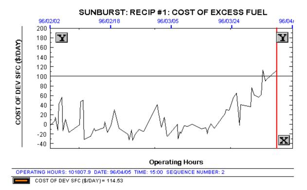
This example illustrates how basic operational data can be turned into useful information for making economically driven decisions. The figure shows the trend of something called "cost of deviation in specific fuel consumption". In other words, this is a measure of the cost of wasted fuel for this engine. Any deviation above zero is, theoretically, an excess cost.
