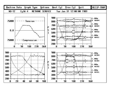
This data can reveal problems such as: leaking valves, leaking rings, excessive HP losses, rod overload, lack of sufficient rod load reversal, crosshead looseness, poor valve dynamics. Some application software is available to assist with detection of problems and to provide some economic measures, such as the excess cost caused by a leak.
