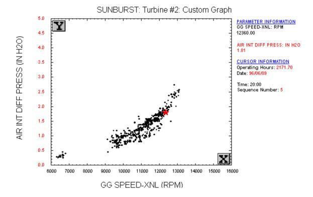
Note that there is potential to go a step further. We should be able to estimate from existing data the amount of efficiency loss for a given increase in intake pressure drop. This would enable the calculation of extra fuel cost, thereby supporting an economically driven decision on filter cleaning/replacement.
