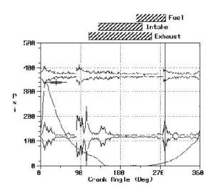
Power cylinder condition and performance can be evaluated from filtered vibration readings and in-cylinder pressure versus crankshaft angle. High speed engines (900 RPM and up) generally do not have provision for measuring firing pressures, so vibration patterns are used to evaluate mechanical condition. In the example at the left there is a pressure-time curve, a filtered vibration pattern (lower) and an ultrasonics pattern (upper).
