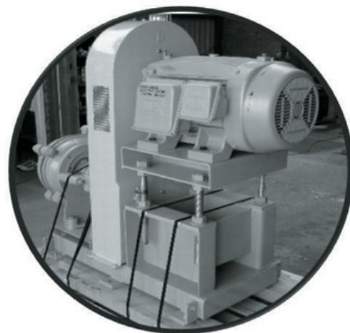
Fig. 11: Slurry pump, motor mounted on platform about pump
