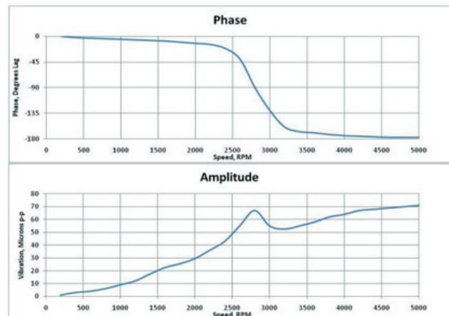
Fig. 2: Idealised bode plot of vibration amplitude and phase vs. speed
