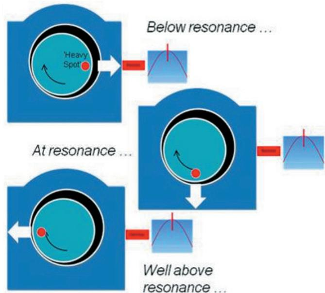
Fig. 1: Phase lag below, at, and above resonance
