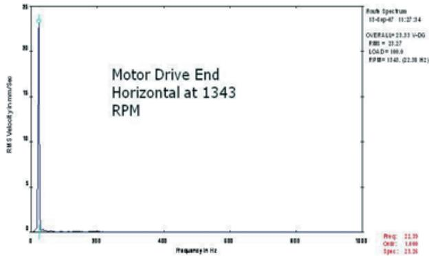
Fig. 12: Motor DE horizontal at 1,343 rpm
