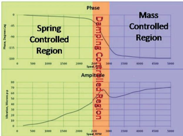
Fig. 9: Bode plot with overlay marking spring, damping, and mass controlled regions
