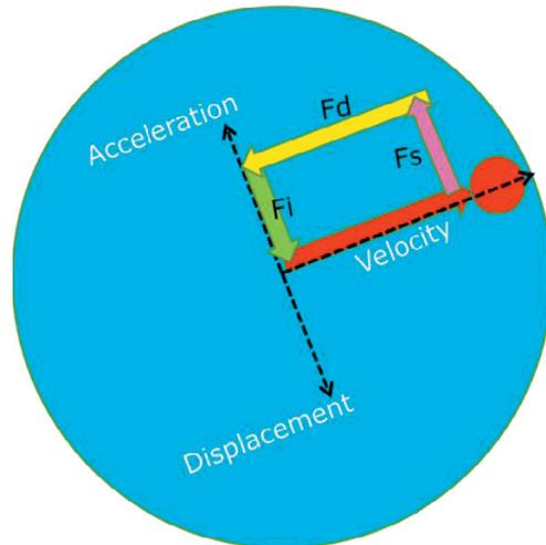
Fig. 7: Force vectors, speed equal to natural frequency
