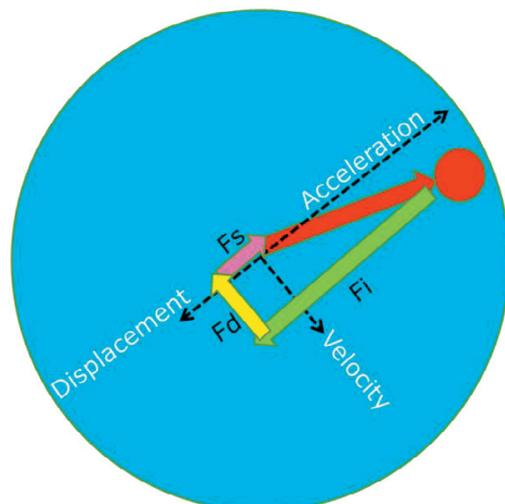
Fig. 8: Force vectors, speed well above natural frequency
