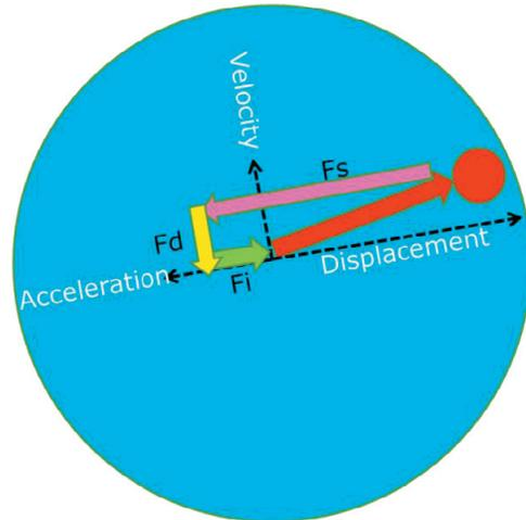
Fig. 6: Force vectors, speed well below natural frequency
