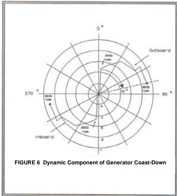
**FIGURE 6** Dynamic Component of Generator Coast-Down
