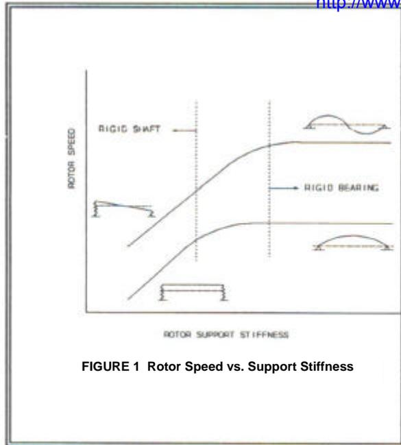
FIGURE 1 Rotor Speed vs. Support Stiffness
