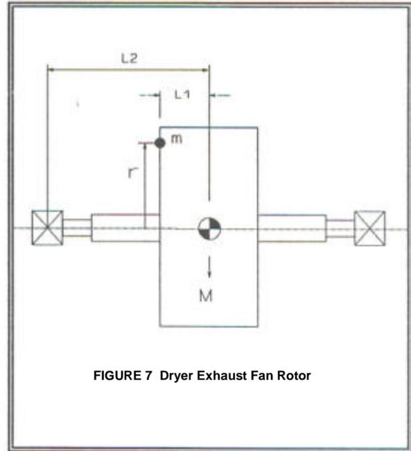
**FIGURE 7** Dryer Exhaust Fan Rotor
