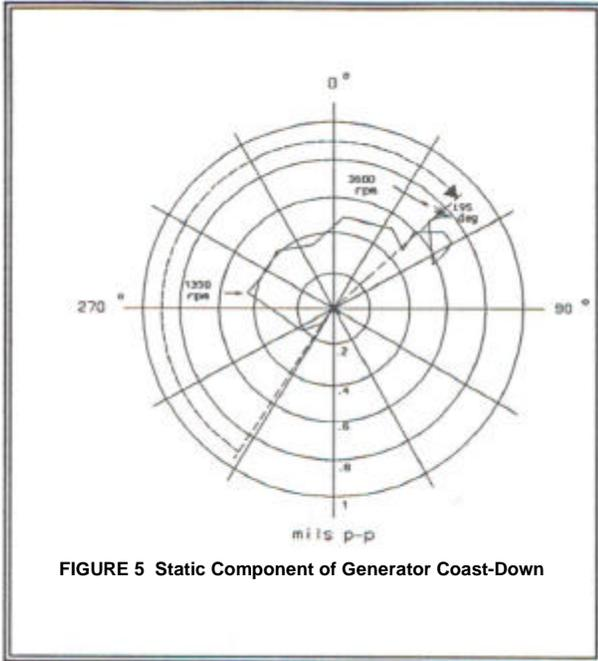
**FIGURE 5** Static Component of Generator Coast-Down
