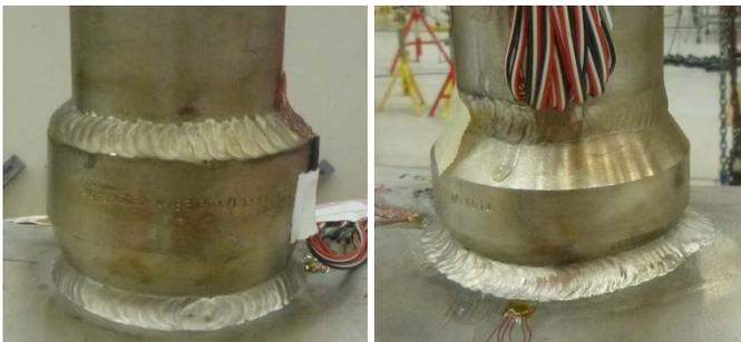
**Figure 7:** Sockolet (LEFT) and Butt weld Pipet (RIGHT) NPS2x20 SBC.
