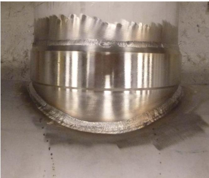
**Figure 6:** Butt weld Pipet tee (NPS 12x20)
