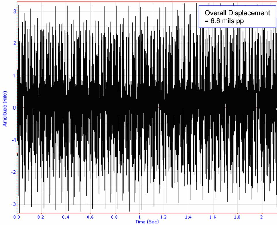
**Figure 8. Velocity Time Waveform Integrated to Displacement with 1x and 2x Filtered Out**
