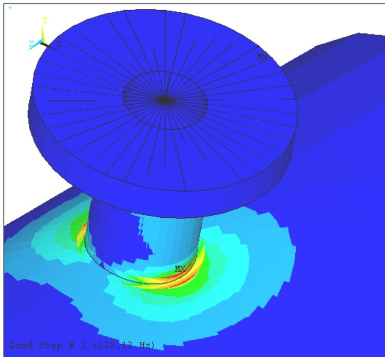
Figure 6. FE Model of Inspection Nozzle - First Order Mode Stress Distribution
