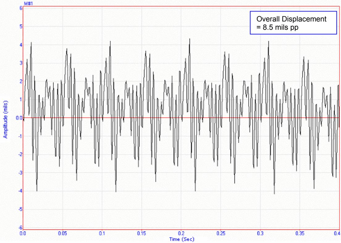
**Figure 7. Velocity Time Waveform Integrated to Displacement**
