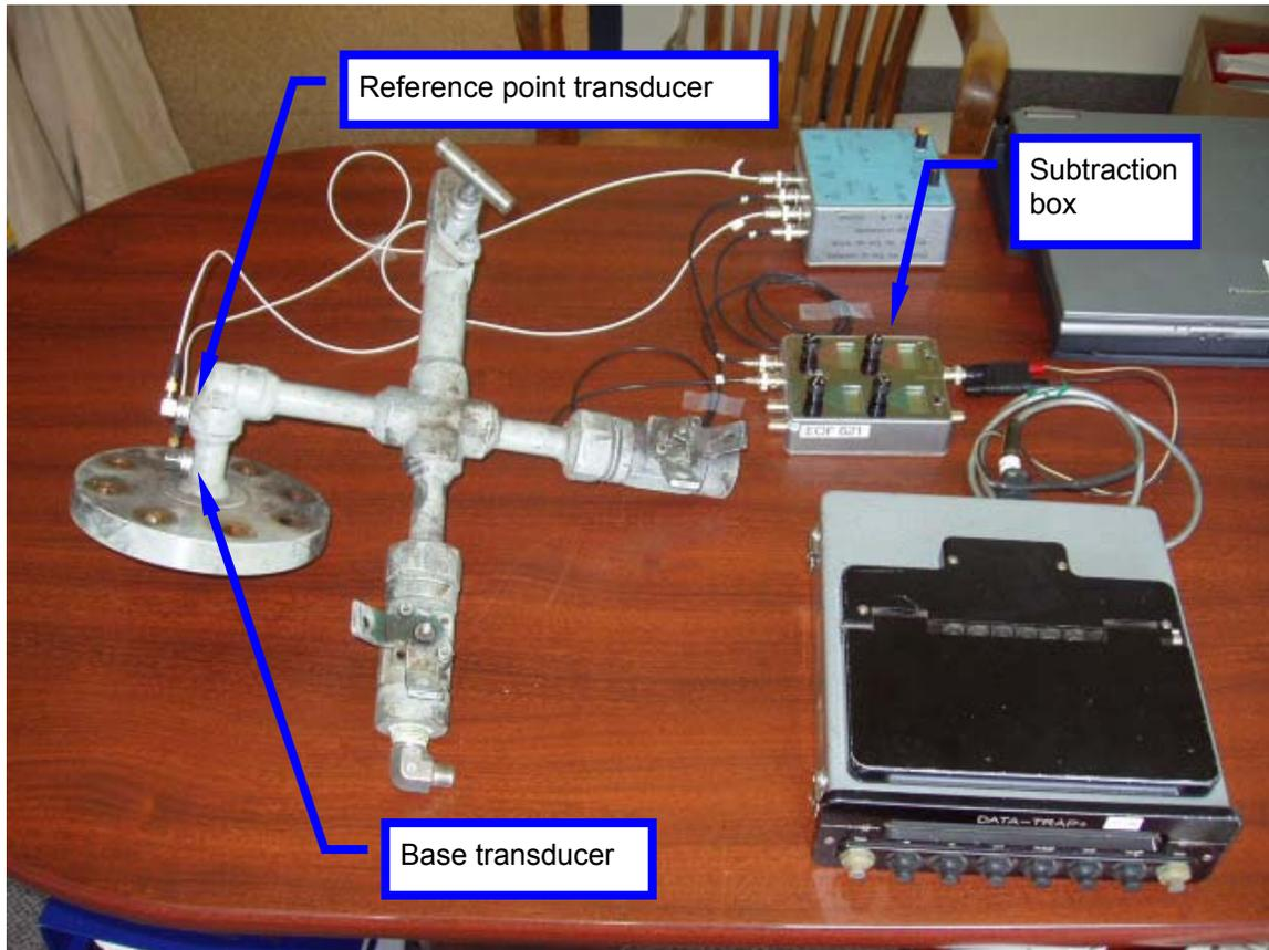
Figure 10. Analysis Setup to Measure Relative Vibration between Base and Reference Point
