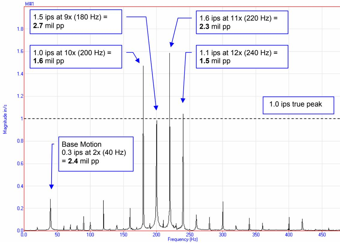
Figure 5. Inspection Nozzle - Spectrum of Velocity Time Waveform
