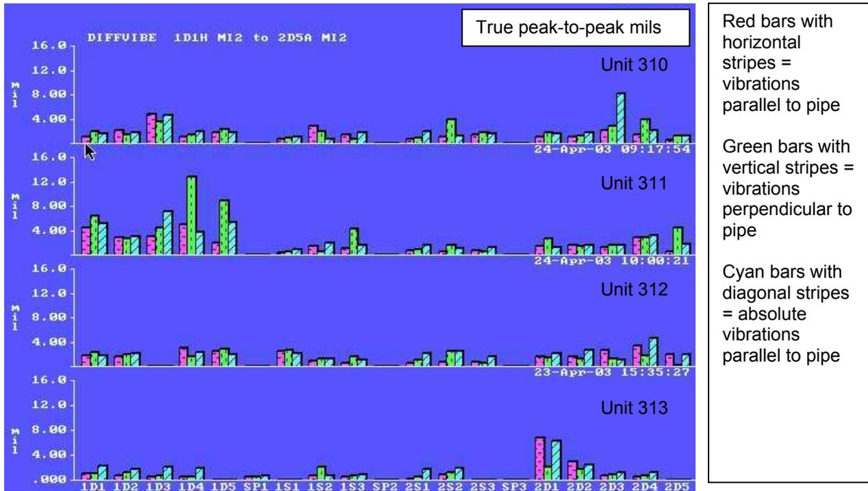
Figure 9. Profile of Vibrations on Small-bore Appendages at Multiple Locations
