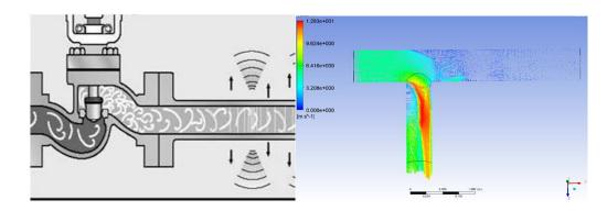
• Turbulence is generated in fluid flowing in piping, leading to vibration with frequency ranges up to 200 Hz
