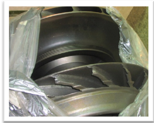
Figure 1: Centrifugal compressor damaged during surge event
